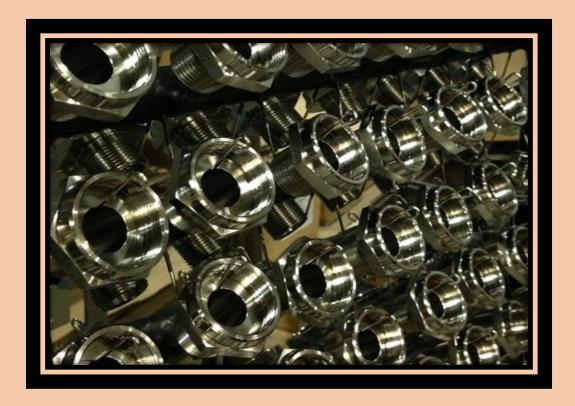
This forms a thin and strong layer of protection that is chemically bonded to the substrate metal. Next, the surface receives a chromate conversion coating, further protecting the thin layer of zinc and nickel.
